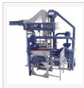
Hulling, polishing and size grading set for small growers and millers
